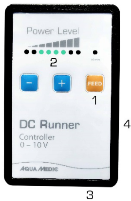
Abb. 2: DC Runner Controller
