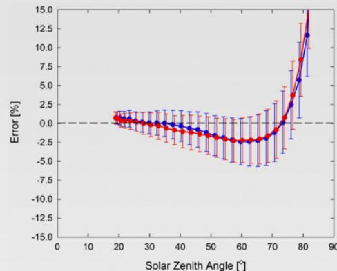
Mean cosine response of twenty-three MQ-210 quantum sensors (**error bars represent two standard deviations above and below mean**). Cosine response measurements were made by direct side-by-side comparison to the mean of four reference thermopile pyranometers, with solar zenith angle-dependent factors applied to convert total shortwave radiation to PPFD. Blue points represent the AM response and red points represent the PM response.
