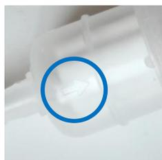
Make sure the tube is pushed all the way up to the filter housing. The filter connection sockets have a slightly larger diameter than the inside diameter of the sample water tube. This is purposely done to prevent the tube from getting disconnected.
