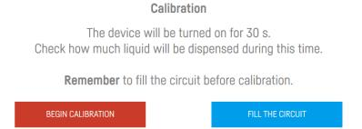
9. The device should be calibrated right after the set up procedure, so that the dosing process is carried out appropriately and the pump is able to correctly indicate the amount of liquid poured to the tank. Before starting the calibration procedure, prepare a container for the liquid poured during the process. During calibration, the device activates the pump for 30 seconds and then automatically deactivates it.
