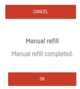
After the specified period of manual refilling expires, the pump returns to the previously configured cycles.
