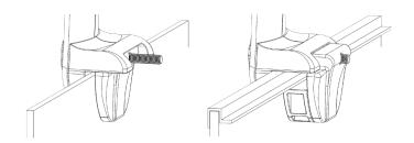
3. Choose appropriate Sliding Rail for desired front to back position
