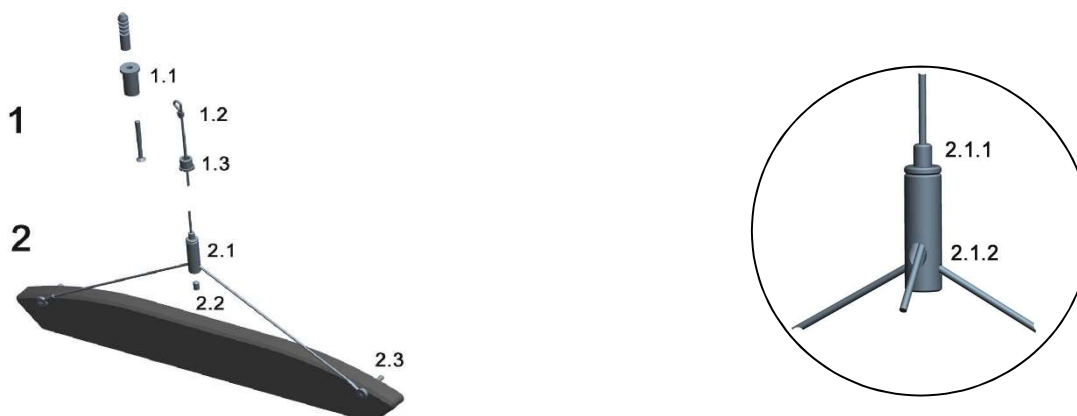
Pict. 1: Steel wire suspension aquafit 2 (art.-No. 80401)
