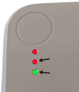
Fig. 2b: The two lower LEDs must flash simultaneously if you want to connect directly to the pump.
