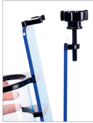
Install the inside plate with the collection cup holder onto the other inside plate.
