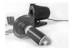
The ceramic shaft is very sensitive and may break immediately if bent.
