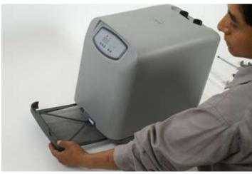
Pull upwards on rear of chiller housing, loosening it on the frame of the chiller.
