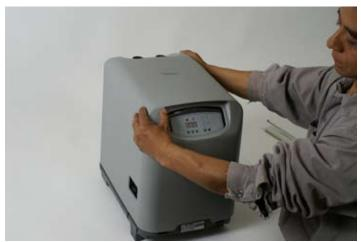
After verifying the UV Lamp is working, turn chiller off and unplug power cord. Lower housing over chiller.
