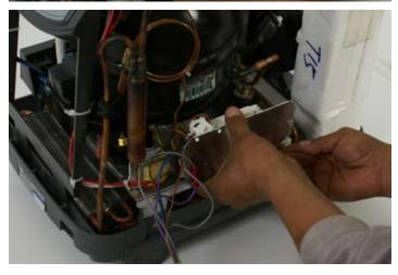
Line the holes in the ballast mounting plate with the holes in the strut supporting the compressor.
