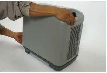
Insert fingers between housing and frame of the chiller at the front. Once fingers are between frame and housing, lift upwards.
