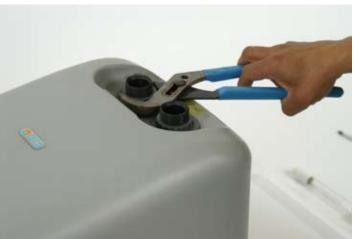
Use channel lock pliers or similar to loosen plastic nuts holding the housing in place. It is not necessary to grip nuts tightly, a loose grip will help prevent scarring of plastic. If desired, a piece of duct tape may be used to cover the teeth of the channel lock pliers to prevent scarring of the plastic nuts.
