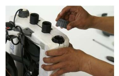
Unscrew and remove ring nut over UV port.
