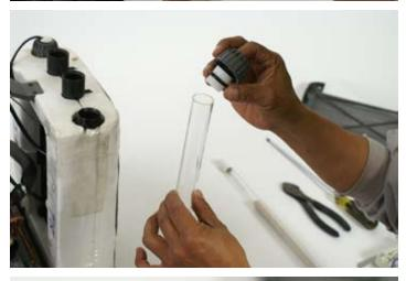
Remove plug and o-ring from ring nut.
