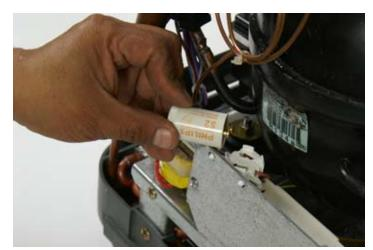
Mount UV starter onto the ballast by inserting pins into slots and rotating clockwise 1/4 turn.
