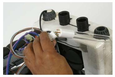
Take UV lamp and insert pins into 4-pin connector on wiring harness.
