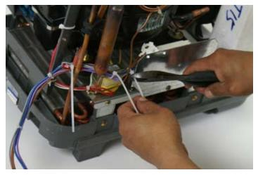
Use zip ties to gather wires together. Clip excess plastic from zip ties with wire cutter.
