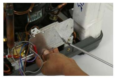
Attach the ballast by screwing the ballast onto the strut supporting the compressor.
