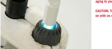
CAUTION: Turn off chiller after checking lamp - Leaving chiller on with no water flowing will cause the unit to overheat.
