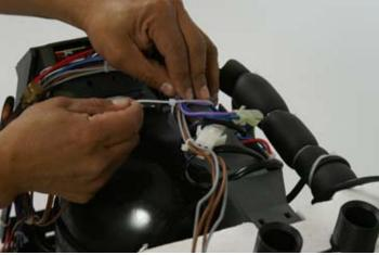
Use zip tie to fasten wiring harness to support strut.
