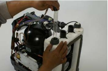
Insert UV lamp into quartz sleeve.
