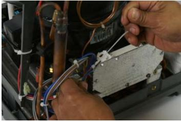
Pull the wiring harness forward and attach the harness to the ballast mounting plate with a zip tie.
