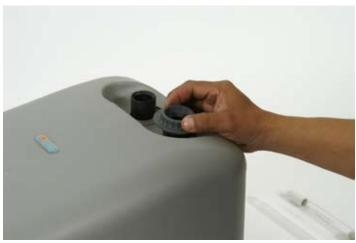
Once loosened, manually remove the plastic nuts.
