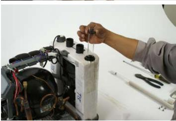
Insert quartz sleeve into heat exchanger until o-ring seats into outlet lip. If you encounter resistance while inserting the quartz sleeve, gently turn sleeve and apply very slight force.
